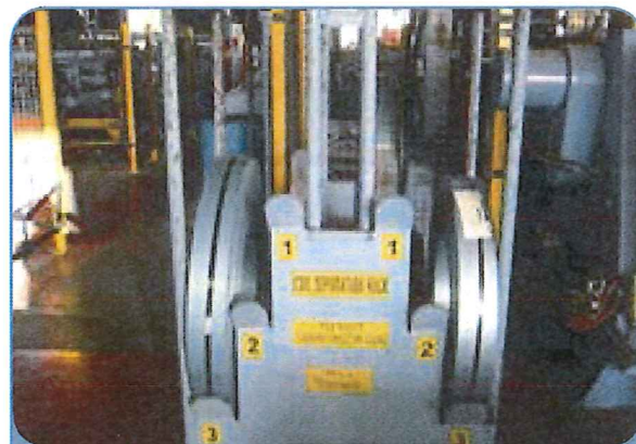
Figure 2: A rack used for separating narrow coils
