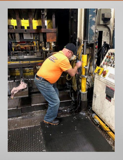
Remove Lockout-Tagout from Power Supply
