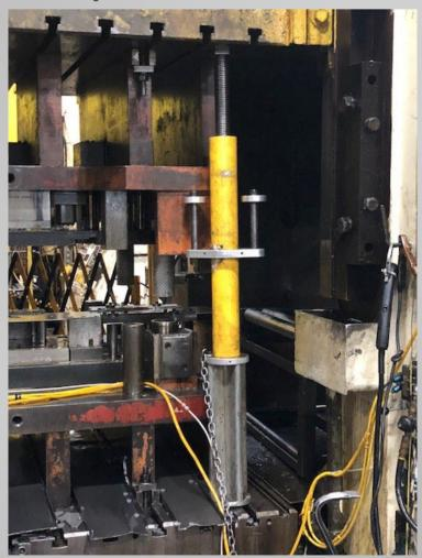
Apply Lockout-Tagout to the Power Supply
