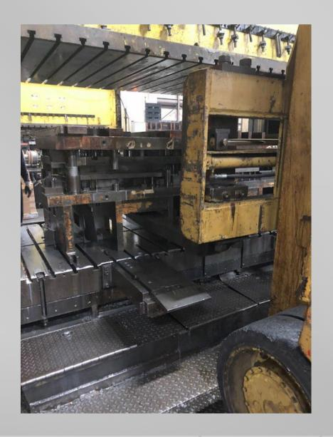
Use the proper tow motor to pull the die out of the press
